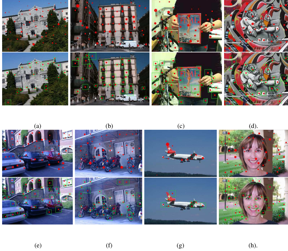
Figure 4.3.1: In each figure (a)-(h). Top row: scale-invariant kernel placement. Larger circle means higher density of converged kernel samples. Bottom row: good kernel regions with appropriate scale selection after pruning texture regions.
